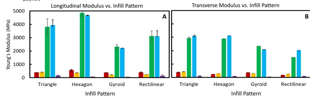
Figure 3. (A) Longitudinal and (B) transverse moduli versus infill patterns for scaffolds with 50% theoretical infill prepared using a variety of polymers.
