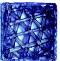
Figure 8. PCL scaffolds with 50% triangle infill.
