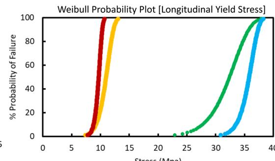
Figure 5. A failure probability graph for 50% triangle infill scaffolds.
