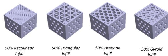
Figure 1. CAD design for 3D printing polymer scaffolds.
