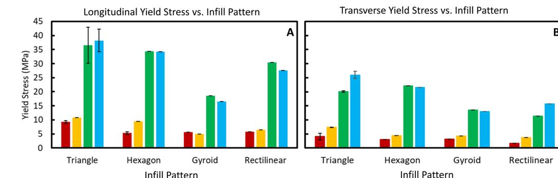
Figure 2. (A) Longitudinal and (B) transverse yield stresses versus infill patterns for scaffolds with 50% theoretical infill density prepared using a variety of polymers
