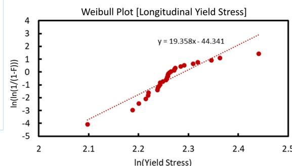
Figure 4. Weibull plot for longitudinally compressed PCL scaffolds (50% triangle infill, shown as an example).
