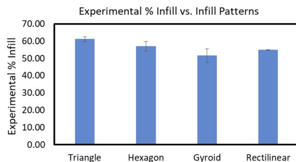
Figure 6. Experimental percentage infill comparison of various 50% geometric patterns (triangle, hexagon, gyroid, rectilinear) for PCL scaffolds.
