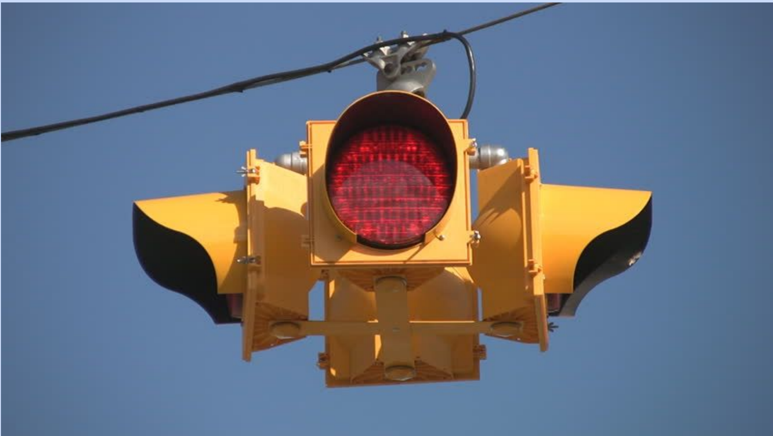
Fig. 2: Single flashing traffic light. Due to the lack of other sequential lights, drivers are unable to use position for reference to determine the color of the light.
